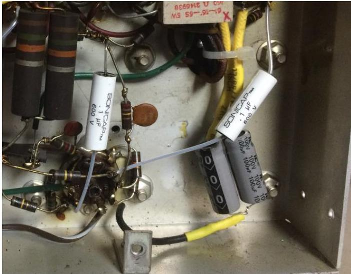
2. Replacing with independent caps under chassis
